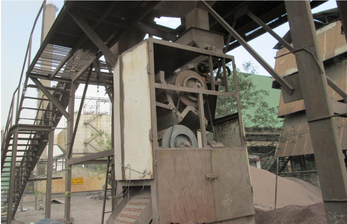
Photo 4: Drum type magnetic separator is used at plant to separate iron from bed ash. This will help to avoid rise in iron in solids inventory in the furnace. This is applicable for pyrite containing coals.
