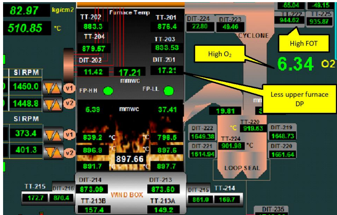
Photo 2: The upper furnace DP is hardly 17 mmWC. The cyclone outlet temperature is 936 & 945°C even with O 2 at 6.34%. The cyclone had not been performing well or the solids input from fuel had been less. It is net retention effect of addition, depletion of fine solids to furnace.
