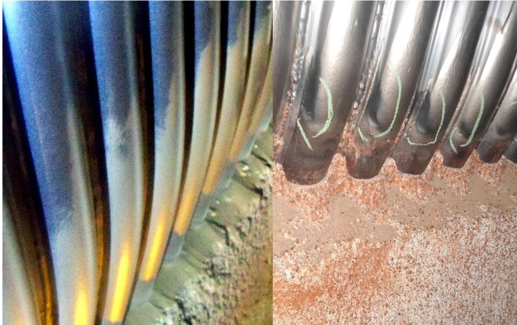
Photo 19 & 20: The above photo shows the erosion of excess refractory constructed at kick off zone. As the projecting refractory acts a brake for falling material, the tubes above get polished / eroded.
