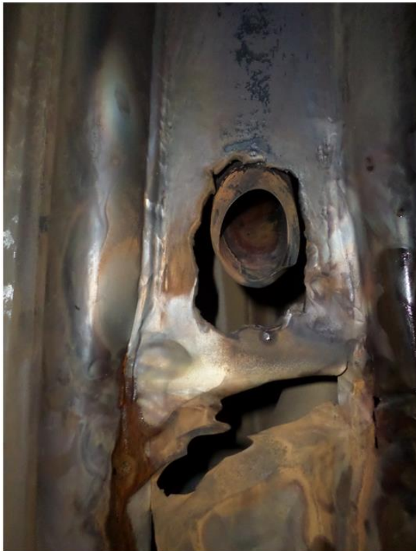
Photo 32; Figure 21: The top photo shows the erosion of tubes when there is an instrument tapping penetration in the panel. A thermocouple at mid of furnace is not required for CFBC furnace.
