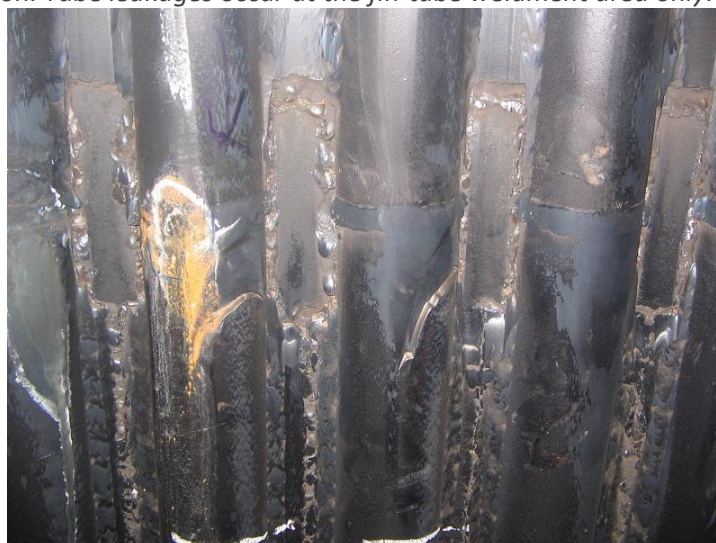
Photo 24: The left side photo shows the haphazard erosion pattern experienced at tube butt / fin butt weld zone.
