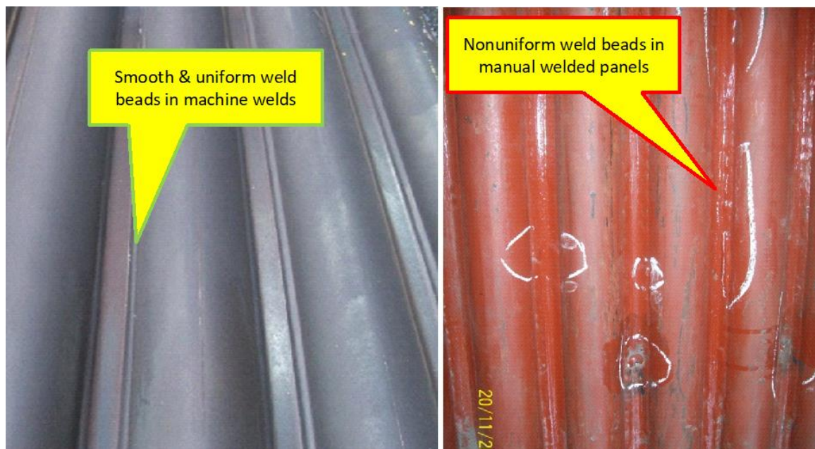
Photo 33 & 34: The difference between panels made by manual process and automat can be seen here. The nonuniform weld beads would cause localised erosion problem.
