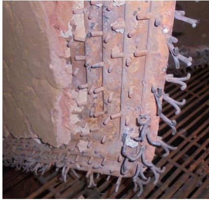
Photo 23 & Figure 14: Photo shows the refractory spalling due to excess refractory. The figure shows the refractory desirable for erosion protection of the outer most tube of wingwall evaporator / SH bottom / bend section. Long anchors are not required at all.
