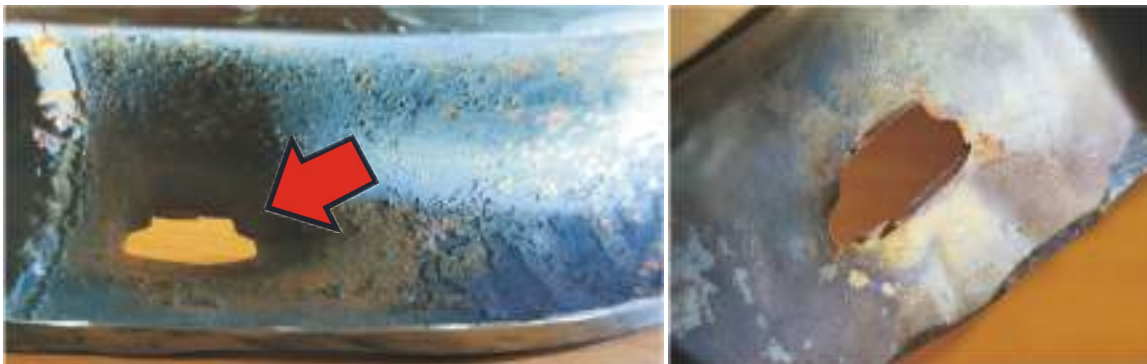
Photo 21 & 22 : The failed furnace tube near burner zone shows iron oxide deposit inside. There is a weld which can easily allow a deposit of suspended iron. The failed edge is typically a under deposit corrosion type.
