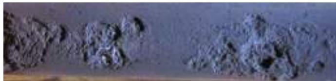
Figure 13: Water side corrosion
