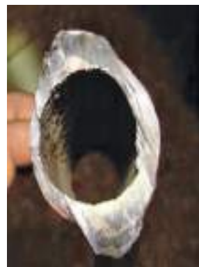
Figure 14: FAC- Economizer inlet stab joint pipes thickness is reduced
