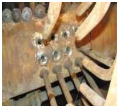
Figure 14: FAC- Economizer inlet stab joint pipes thickness is reduced
